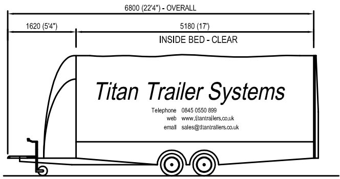
SIDE ELEVATION WITH CANOPY CLOSED
